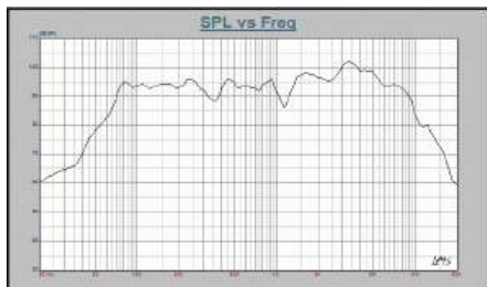
AЧХ (1Вт/ 1м) / RESPONSE CURVE (1w/1m)
